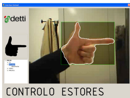
Figure 11. The application interface installed in the “House of the Future”. The recognized static pose is presented to the user on the left, and the triggered action is indicated below (opening the window blinds).
