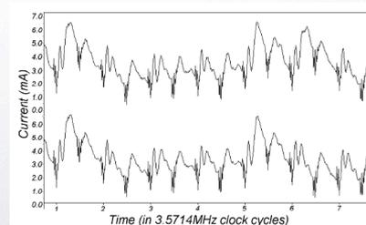
Figure 3: SPA trace showing individual clock cycles.
