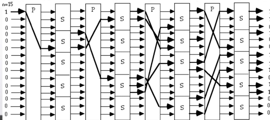
Fig 2.3 - Substitution-Permutation Network, with the Avalanche Characteristic
