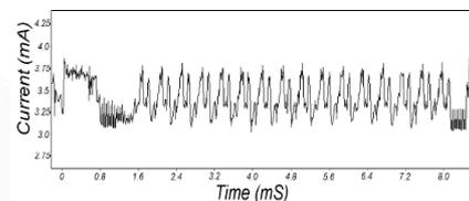
Figure 1: SPA trace showing an entire DES operation.
