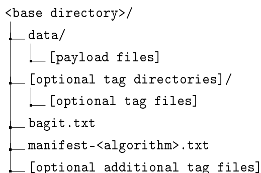
Figure 16: Basic bag structure.
