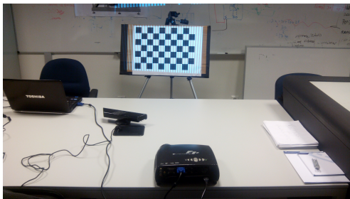
Figure 36: Two examples of positions between the sensor and the projector. In the left they are placed in a table to project against the wall. In the right they are placed in the ceiling for top-down projection.
