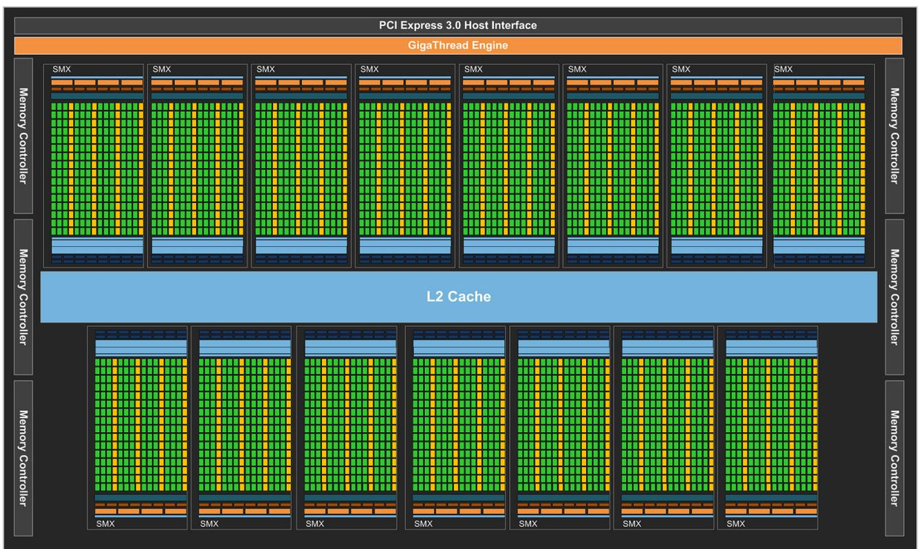
Figure 7.: Kepler architecture - full chip block diagram <sup>1</sup>
