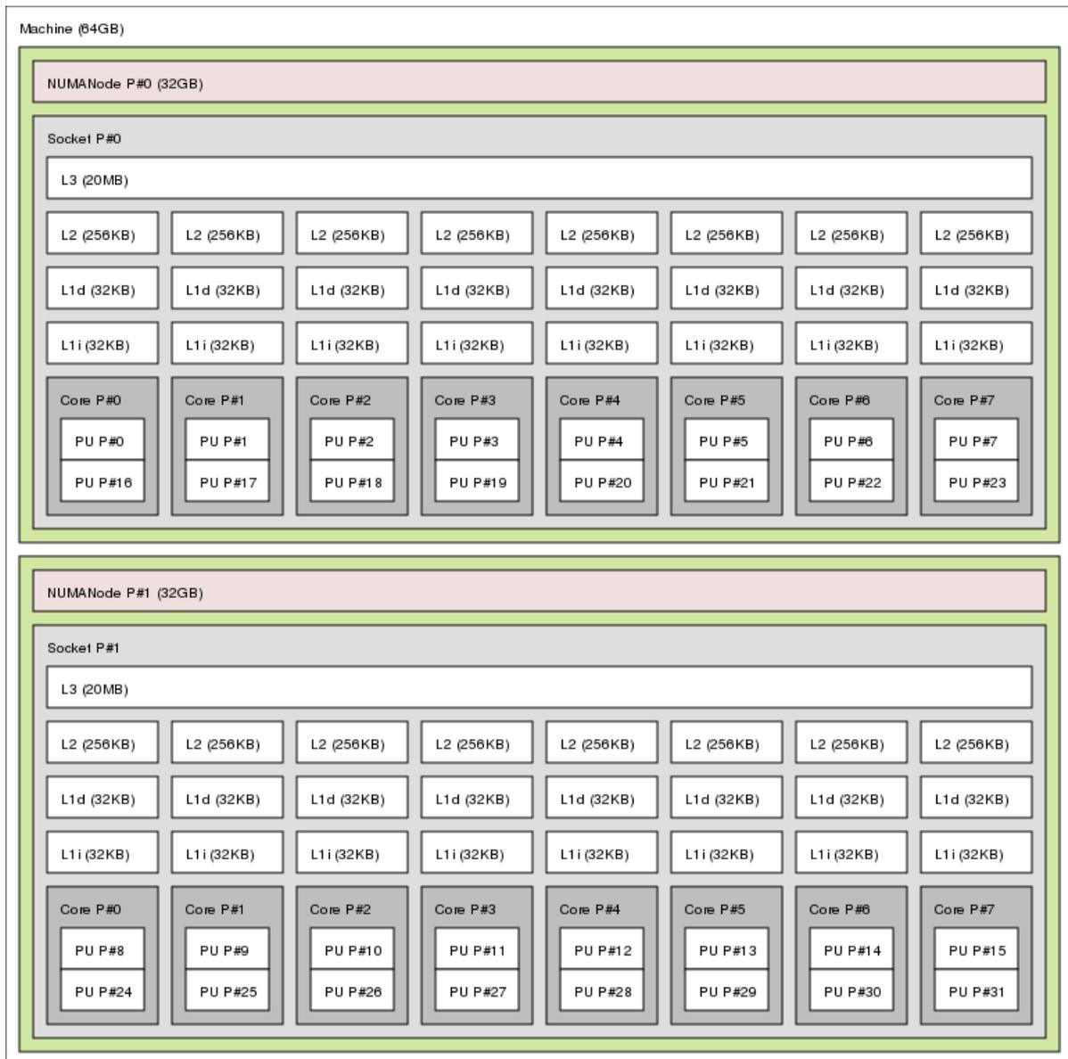
Figure 6.: Shows the node topology used in the experimental setup
