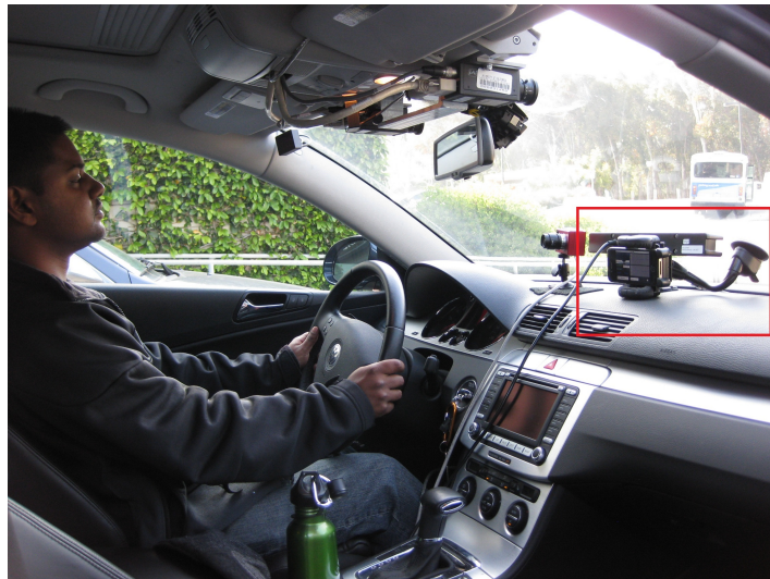
Figure 16.: Position of mounted mobile device in Johnson et al. (2011).
