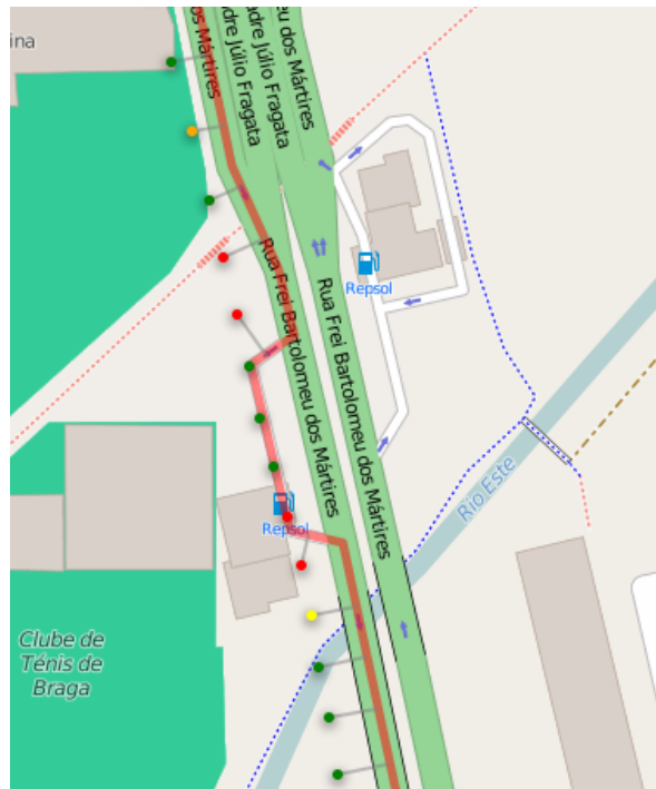
Figure 24.: Case where the map matching inferred incorrectly the path.
