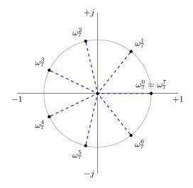
**Figure 5.1:** The values of the 7th complex roots  $\omega_7^0, \ldots, \omega_7^6$  in the complex plane, where  $\omega_7^7 = e^{2\pi \frac{j}{7}}$  is the principal 7th root of unity.
