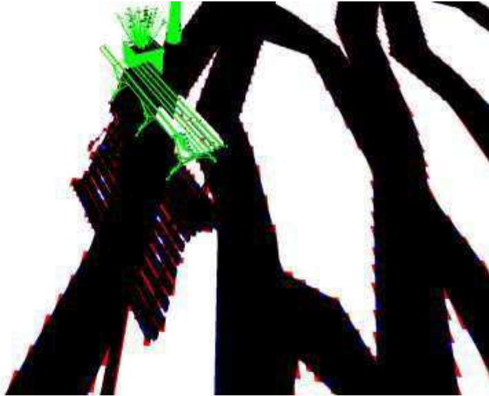
Figure 43 - Average Case Result for BGSM; Red pixels represent the Shadow - Incorrect; Viewport Size: 1920x1080; Shadow Map Size: 4096x4096.
