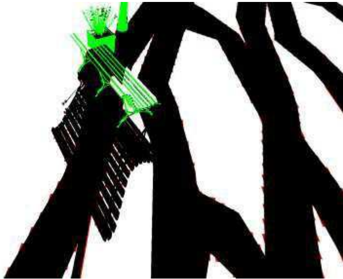
Figure 52 - Average Case Result for CSM without Adjacency; Blue pixels represent the Light - Incorrect and the Red pixels represent the Shadow - Incorrect; Viewport Size: 1920x1080; Shadow Map Size: 4096x4096.
