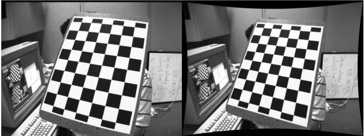
Figure 7: Example of an uncalibrated (left) and calibrated (right) image of a chessboard pattern. As we can see, the curves on the left were adjusted to look like lines on the right.
