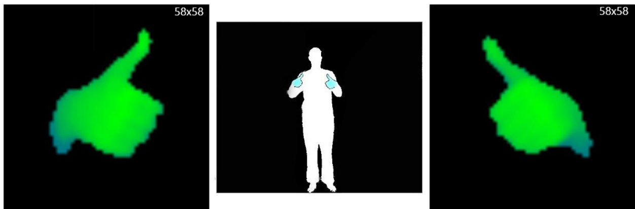
Figure 30 – Depth data input for the both hands. At the left side is the left hand and at the right side the right hand. The middle image is the original depth input after applying the background extraction. At the top right corners it is possible to see the original size of the hand image. The colour representation is merely visual since the input for depth values varies from 0 (the sensor) to the max range the sensor can infer depth (accurately is only 4.5 m, hence 4500).
