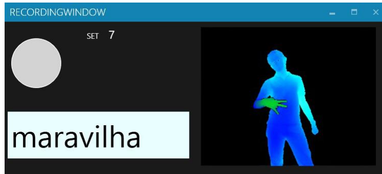
Figure 10 – Sign recording helper window. The purpose of this window is to help the signer to know what sign to perform and when to perform it.
