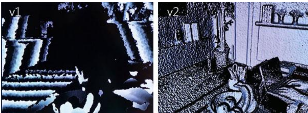
Figure 3 – Kinect versions depth comparison. The left image corresponds to the first version of the Kinect sensor, released in 2008, while in the right it is the same scene with the new Kinect One sensor. (Microsoft, 2014a)
