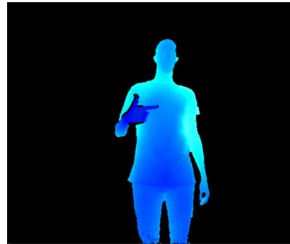
Figure 21 – Kinect sensor depth input after applied the background subtraction. With background subtraction - the body silhouette becomes the only visible object as it is the only object that moves in the sensor field of view.
