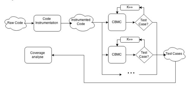
Figure 27 Test case generation following the token methodology
