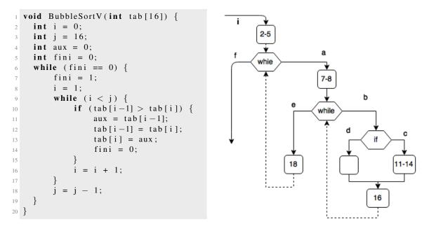
Figure 30 Bubble sort function
