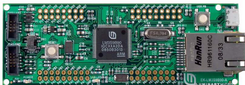
Figure 4.2: LM3S9B90 Evaluation board
