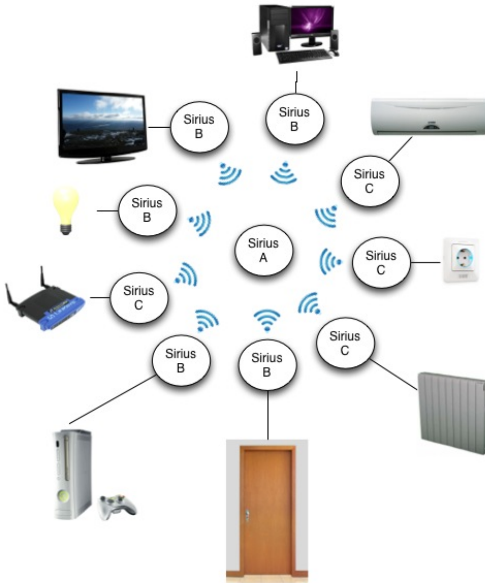
Figure 4.2: A network based on N-Core devices connected to some home appliances and doors
