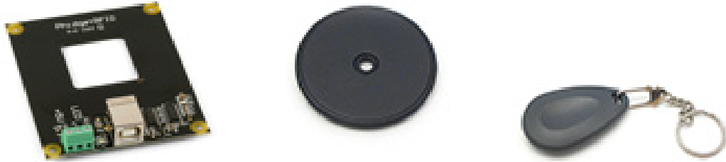
Figure 4.4: Phidgets RFID tag reader (To the left), RFID black tag (On the center) and RFID keychain black tag
