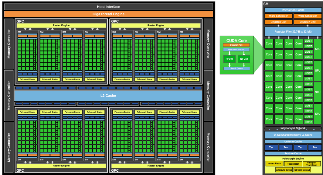
Figure 2.2: Nvidia Fermi GF100/GF110 architecture. Chip diagram on the left and SM diagram on the right. (Source Nvidia)
