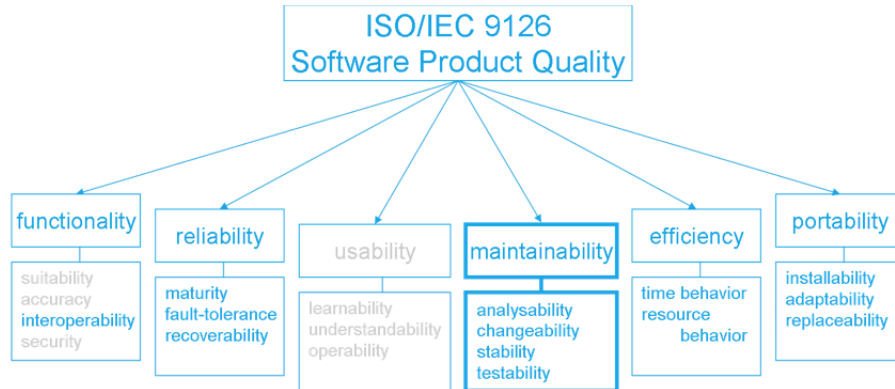
Figure 2.5: The SRA process focuses on the technical aspect of the software product, in particular on its maintainability.
