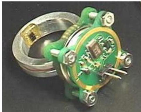
**Figura 4: Protótipo do MIT do "The Ring Sensor - A New Innovative Device for Continuous and Wireless Health Monitoring"**
