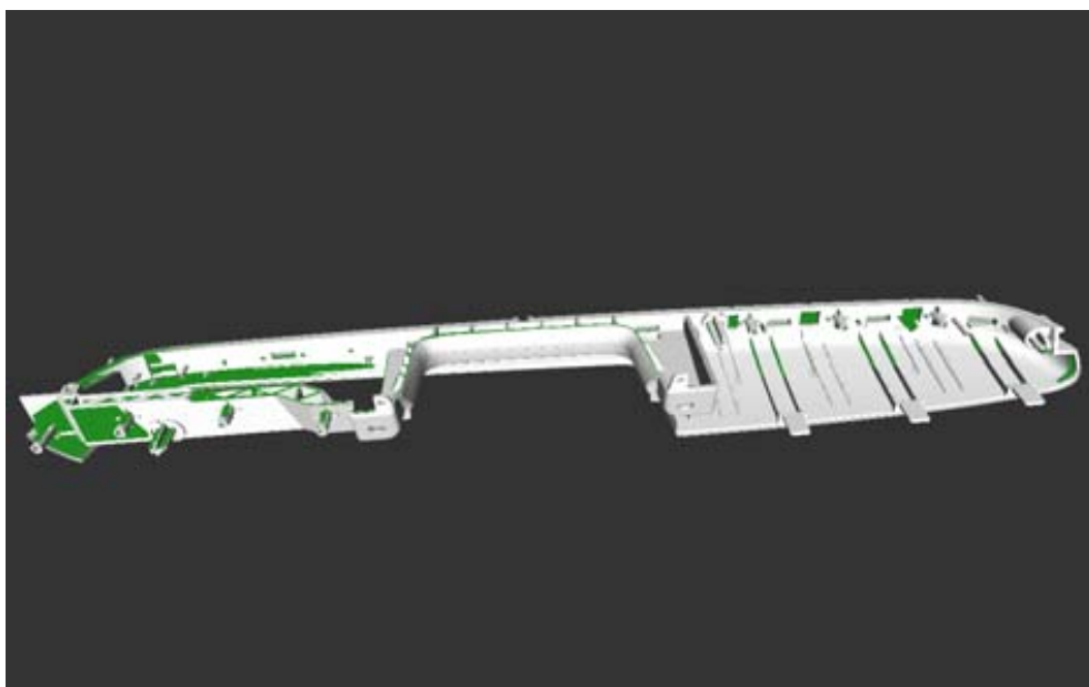
Figure 5.14: The surface (white) and mid-plane mesh (green) of the Door Handle New model.
