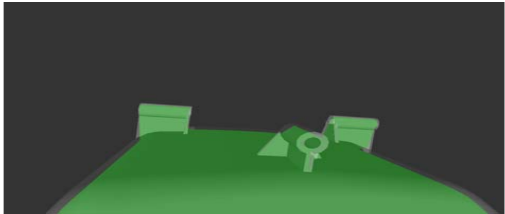
Figure 5.25: Some of the geometric features that form the Door Handle model. As can be seen, the angle formed between the surface (bottom green zone) and these geometric features is, approximately, 90^\circ .
