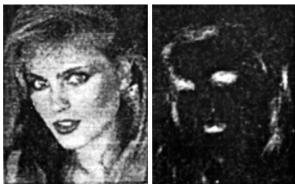
Figure 3.5: A grayscale image and the result of applying a symmetry detector on it. Reprinted from [Reisfeld and Yeshurun, 1995]
