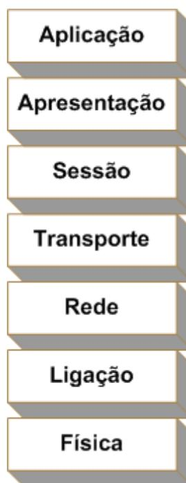
Figura 3: Camadas Open Systems Interconnection (OSI)
