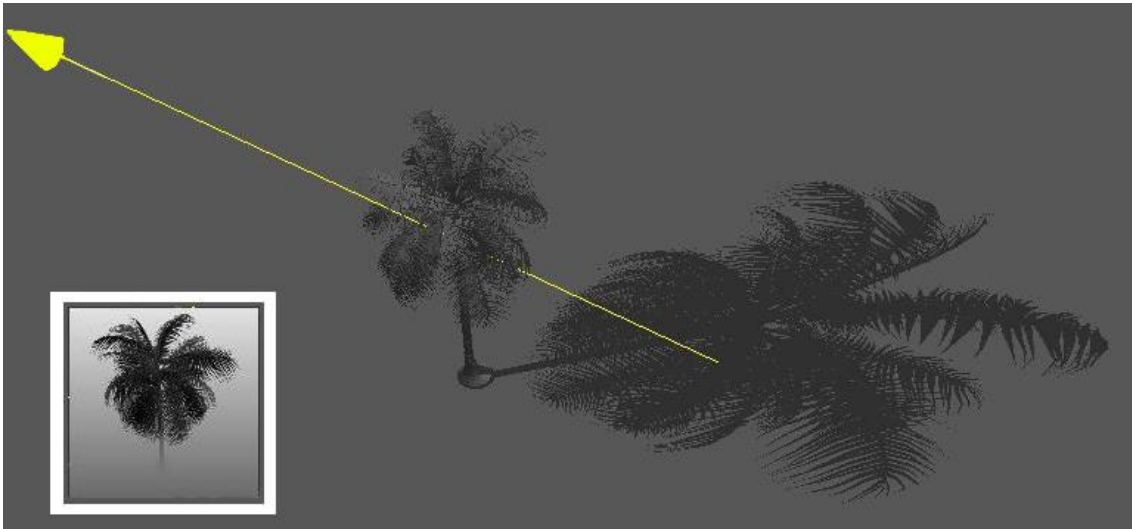
Figure 6: Shadow created with a shadow map. Bottom-left square shows a shadow map created from the light point of view.
