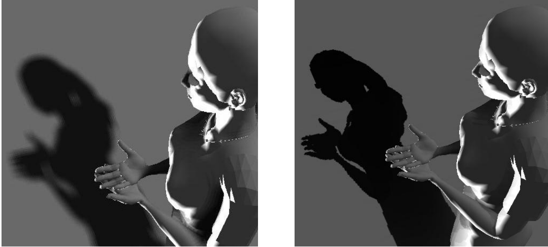
Figure 44: Scene rendered with a 512 shadow map: (left) PCF 4x4 vs. (right) VSM
