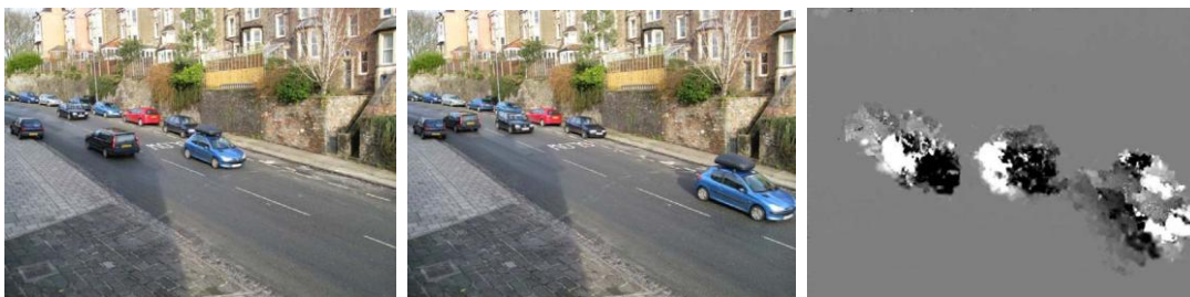
Figura 10 - Image 1; Image 2 ; Hierarchical Lucas-Kanade – horizontal motion
