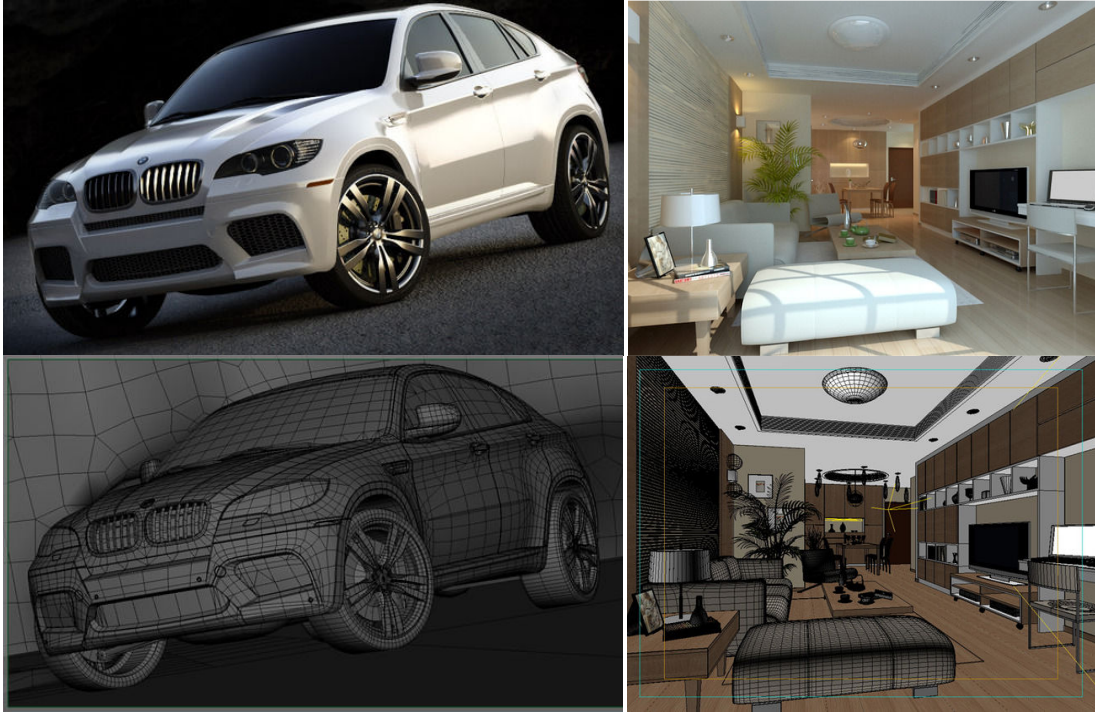
Figure 2-1. Ray Tracing used in Car Styling and Architecture
