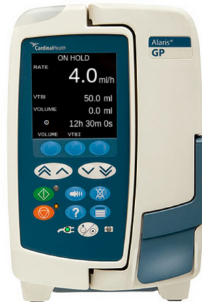
(b) PVSio-web prototype of the AlarisGP pump. The figure shows a snapshot of the prototype executed within PVSio-web.
