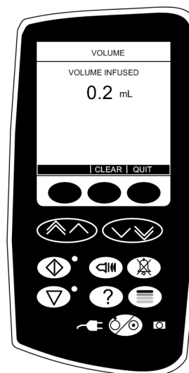
Fig. 4. The same function keys are always shown when top line is “volume”.
