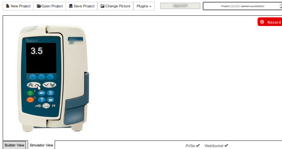
Fig. 4: Example interaction with the PVSio-web simulator: the user clicks on virtual device buttons, and watches feedback on the virtual device display.
