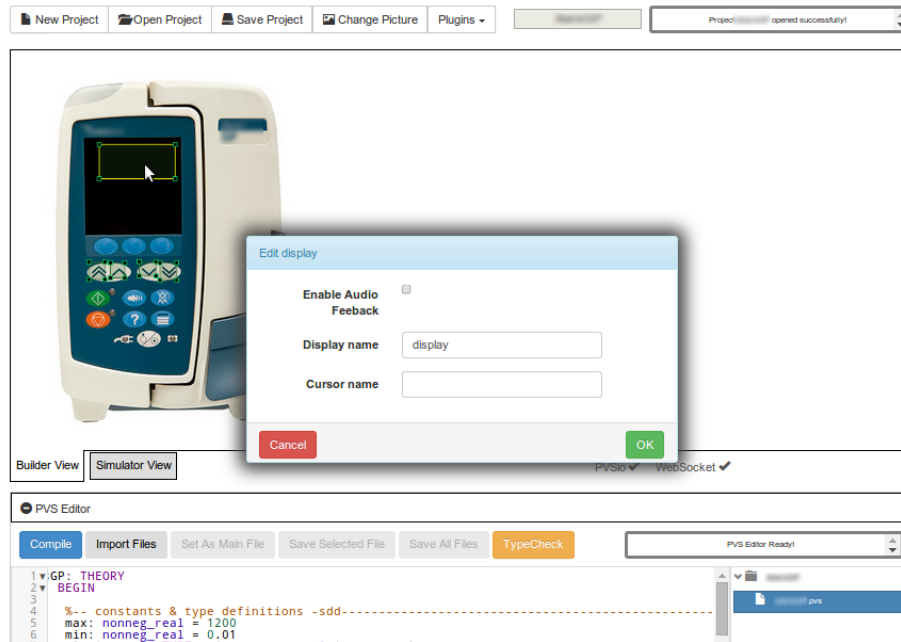
Fig. 3: Snapshot of the graphical editor bundled with PVSio-web. Shaded areas over the picture represent interactive areas for input and output widgets. The form shown upfront allows designers to configure the selected interactive area.
