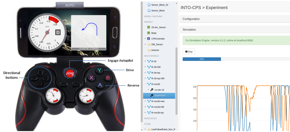
Fig. 4. Screenshot taken during a co-simulation run. The dashboard prototype is on the left. The output of the INTO-CPS co-simulation window is on the right.
