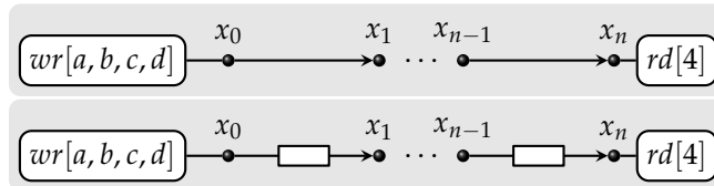
Figure 7.8: Sequences of n Sync channels (above) and FIFO 1 channels (below).
