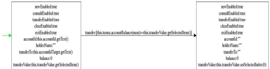
Fig. 6. Part of the JBank state machine
