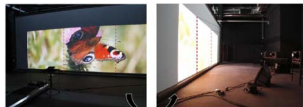
Figure 2. The visualization system in a PowerWall configuration. The red marks delimit the area of projection of each projector. Blending functions are used in order to give the sense of an uninterrupted projection surface.
