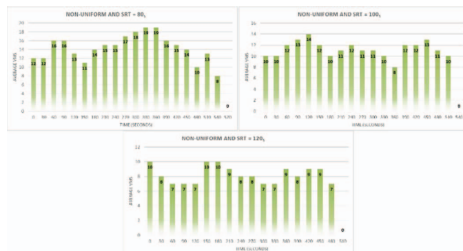
Figure 2. Type 1 Requests (Select-Range): average virtual machines used for workloads randomly arriving between 10 and 60 seconds for the SRTs: 80, 100 and 120 seconds.
