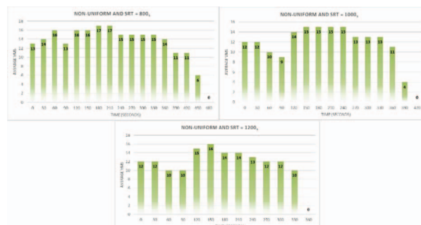
Figure 4. Type 3 Requests: average virtual machines used with workloads randomly arriving between 10 and 60 seconds for the SRTs: 800, 1000 and 1200 seconds.
